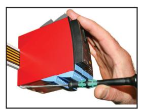
**Picture 1:**By lifting the bottom lock, the device is detached from the DIN rail.
