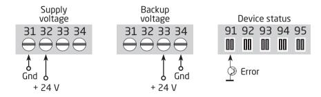
If no backup supply: Place a jumper between pin 32 and 33
